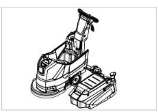
→ Lift up the waste water tank and put it aside.
